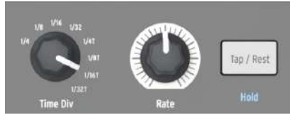
The Time Div encoder, Rate knob, and Tap/Rest button
